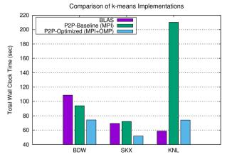
BLAS formulation yields best performance on KNL, despite many more distance calculations than point-to-point (P2P) approach using "acceleration"; slightly slower then P2P distance calculation on SKX.
