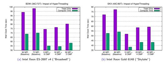
Figure: Comparison of times to cluster the GSMNP LiDAR data set with k = 2000 on the Broadwell (BDW) and Skylake (SKX) Xeon processors for different numbers of MPI ranks and OpenMP threads.
