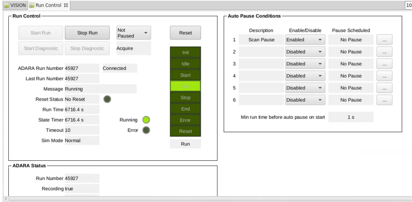
Fig. 4. Screen capture of EPICS based control interface for neutron imaging instrument at SNS.
